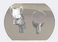
Fit the valve handle over the valve toggle and secure in postion by tightening the screw through the access hole in the top of the handle, complete by pushing the chromefinishing cap in to the aperture.
