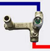
Secure valve block at correct depth accounting for wall finishings, connect hot and cold water feed pipes Refit dock and valve stem protectors to protect during first fix finishing, plastering / tiling etc Hot In
