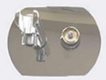
Lubricate the shower dock o rings with plumbers silicone grease then slide the shower dock over the stem and tighten securely in position with the allen screw located on underside of the dock
