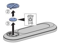
2 Insert a new CR2032 battery. The device beeps (1x) and the blue LED on the lateral control panel lights up for 4 seconds.
