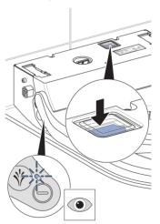
✓ The LED on the lateral control panel flashes/goes out.
