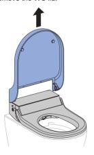
4 Remove the design cover for complete cleaning.
