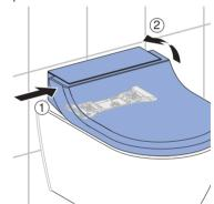
3 Lift the device as far as the removal limiter permits. Clean the gap between the shower toilet and ceramic sanitary appliance.
