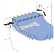
**3** Lift the device as far as the removal limiter permits. Clean the gap between the shower toilet and ceramic sanitary appliance.
