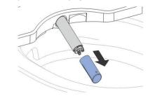
4 Replace the spray nozzle if it can no longer be completely cleaned and descaled.
