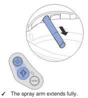
**3** Hold the spray arm firmly and remove the spray nozzle from the front to clean and descale it. Always ensure that the spray nozzle moves parallel to the spray arm.
