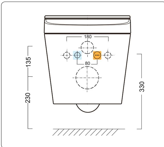
**Utilising wall frames with integrated electricity and water supply**
