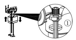
adjust the float upwards to increase the inlet volume; or downwards to reduce the volume
