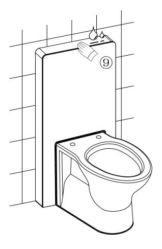
Test half & full flush functions.
