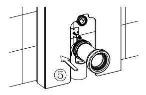
Fit the straight waste pipe in to drainage pipe
