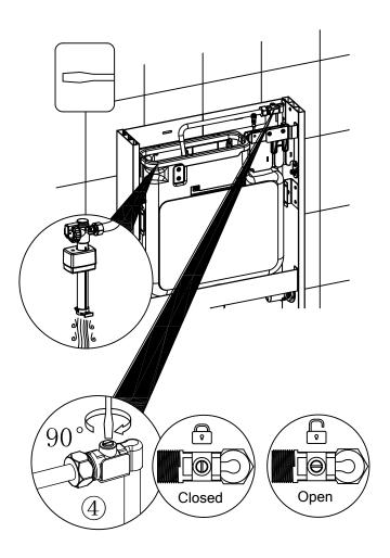
open the valve on flexible hose,and observe whether water supply is normal and if there is any leaking on flexible and cistern.
