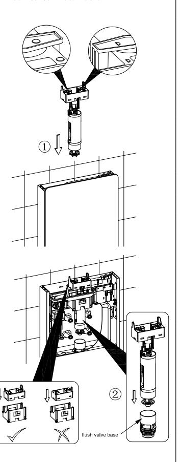
install the flush valve downwards into the cistern body(Mark: make sure the flush valve bottom is aligned with flush valve base. And please make sure flush valve is installed in the shown direction during installation.
