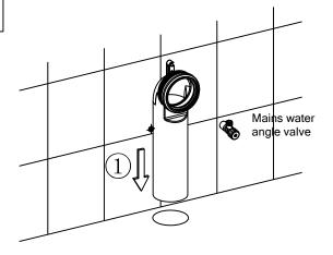
Insert the drain pipe in to the soil pipe foor joint as shown
