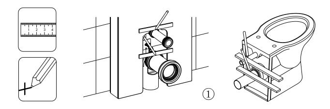
Mark both the Flush and straight drain pipes
