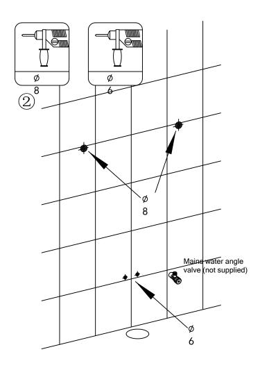
Drilling on marked points(the holes depth must be longer than the expansion nuts length,and the holes diameter is shown above)
