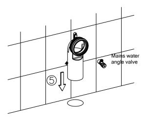
Insert back the drainage pipe into the hole on the floor (make sure it is thoroughly inserted)
