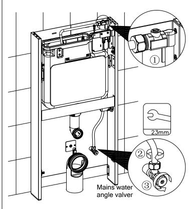
Buckle the flexible hose into the hook on the back panel and then connect the flexible hose to the angle valve
