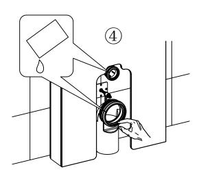
Apply silicone grease to the flush and drain gators
