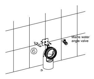
Attache the square back plate securely to the wall
