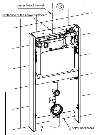
Place the cistern frame up to the wall in the correct correct position aligning the cenet lines on the top and bottom bach board with those previously positioned on the wall and floor
