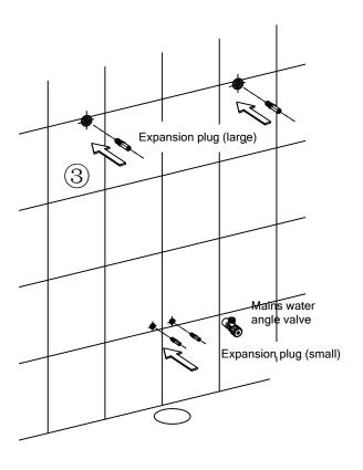
Insert the expansion nuts into the drilled holes.
