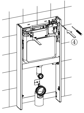
fix the big screws into the expansion nuts on the wall,and lock up the frame on the wall tightly.
