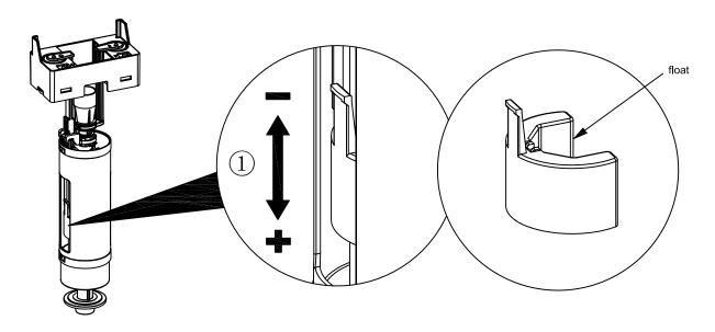
adjust the float upwards to reduce the flush volume; or downwards to increase the volume
