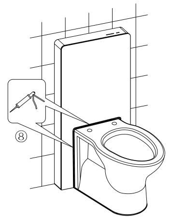
Apply silcone sealant to seal pan ton cistern glass
