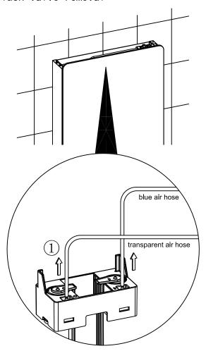
un-connect the air hoses from the air hose holes
