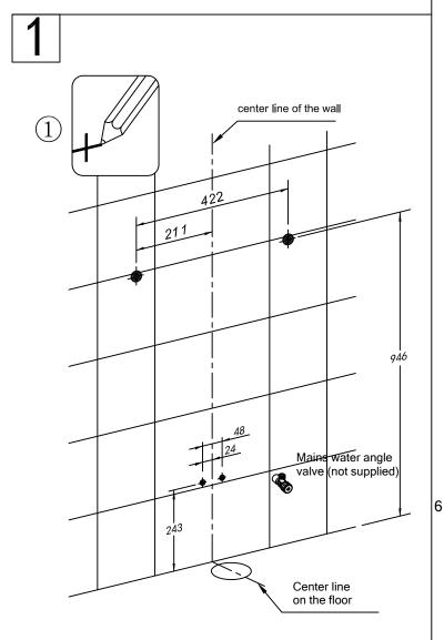
As shown in the picture, drawing up center lines of the ground and wall according to the center of drainage hole firstly, then marking four points on the wall.
