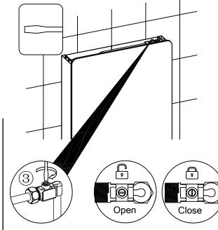
turn off the stop valve on the flexible hose
