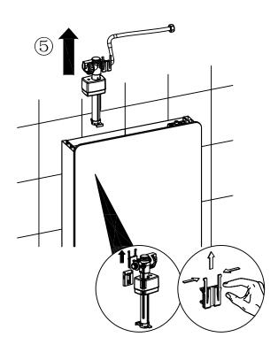
Remove inlet valve lifting upwards
