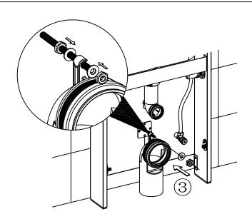
Fix the drainage pipe onto the wall by using square plate.
