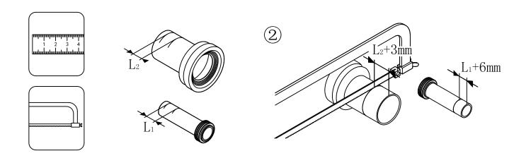
Cut the flush pipe and drainage pipe.
