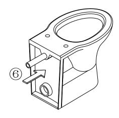
Install the flush pipe onto the toilet.
