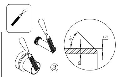
Chamfer and smooth the cut edges on both the flush and straight drain pipes
