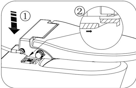
Align the seat cover to the fixing plate
