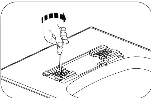
Loosen the bolt in counter clockwise direction by screwdriver
