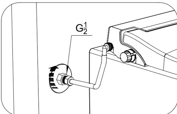
Connect the water supply hose to the water connector on the wall
