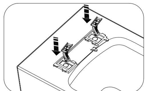
① Assemble hinges and fixing plate according to the figure above
