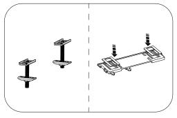
① Assemble hinges and fixing plate according to the figure above
