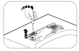
Keep lifting upward the adjustable plate and continue rotating the bolt counter clockwise until the screw is fully removed
