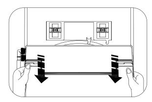
Press the quick release button meanwhile pull the seat cover backward
