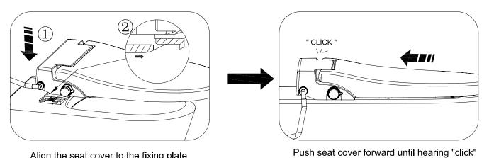
Align the seat cover to the fixing plate
