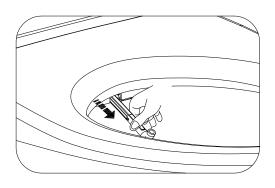
Remove the nozzle regularly for cleaning or replace it with a new one
