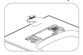
Take out the bolt ,toggle plate, and screw nut, then loosen another hinge
