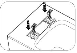
③ Tilt the toggle plates of the hinges and insert the hinges into the toilet mounting holes
