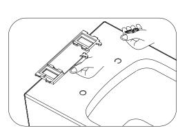
Remove the fixing plate
