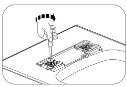
Loosen the bolt in counter clockwise direction by screwdriver
