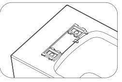
② Install the fixing plate with gaskets on the toilet and align the mounting holes
