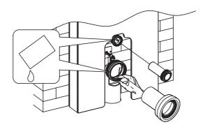
make slant angles on the flush pipes
