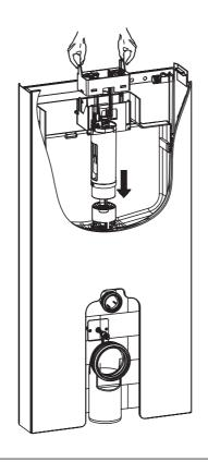
b. place the flush into the cistern, making it align with flush valve base
