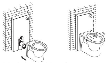
Fix the toilet to the cistern, and adjust it until it is in a proper position.
