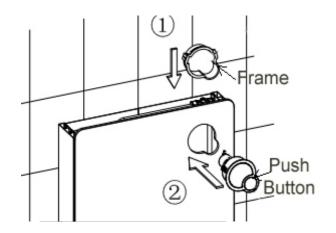
After inserting the push button in the glass insert the two plugs as illustrated
