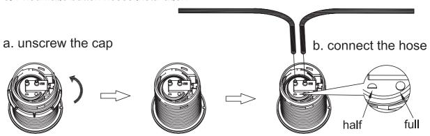
For full flush actuation, connect the transparent hose to the hole marked "o" For half flush actuation, connect the blue hole marked "D"
