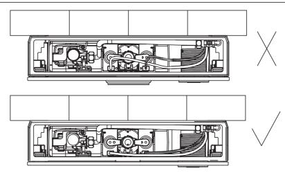
Mark: air hoses cannot be on the upper of the lever, which will interfere with lever's normal working.
