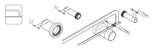
Cut the flushing pipes according to your needs.
