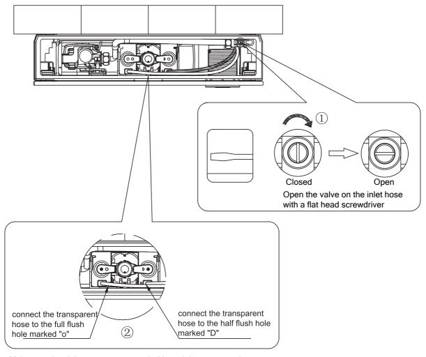
Make sure the air hoses are connected with push button correctly.
