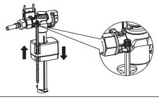
inlet valve maintenance: back cover can be removed to clean the washer if inlet valve cannot stop water or water inlet too slow;
