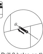
a. Drill 2 holes on the wall accordingly, then place the expansion bolts into the prepared holes
