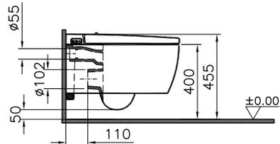
Additional pipe may be required due to wall thickness.
