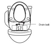
Screw the drain bolt and install the appliance.
