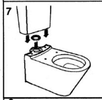
Place rubber seal into pan recess (DO NOT USE SEALANT). Place cistern screws into holes on the inside of cistern, making sure washers are located correctly. Gently lower cistern onto pan locating fixing screws into matching pan screw holes. Secure cistern to pan. Before tightened fully make sure cistern sits square and straight to
