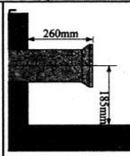
5.Set up waste pipe so that the end of the pan collar extends 260mm from the finished wall.
