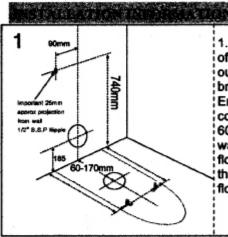
1.Rough in position of water inlet, waste outlet and floor fixing bracket holes. Ensure inlet connection extends 60mm from finished wall. Drill holes for floor fixing bracket then fix brackets to floor.
