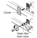
(4) After draining the water, install the water filter drain valve and cover. Insert the water filter drain valve and use a flat-head screwdriver to tighten it securely.
