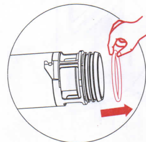
④Take out of the sealed rubber of flush valve, clean or replace it.
