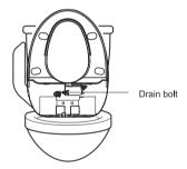
Screw the drain bolt and install the appliance.
