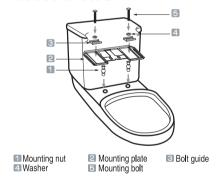
How to attach and detach the unit
